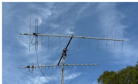
Figure 1 : an UV Yagi antenna specifically designed for receiving satellite
