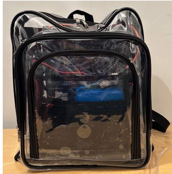
Figure 7 : The FT-991A backpack contains a transceiver, battery, handheld microphone, and antenna.
